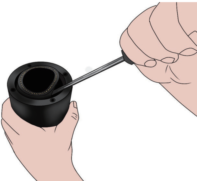
3. Lubricate the outline where the rubber hose contacts the inner wall of the valve body with wrench
