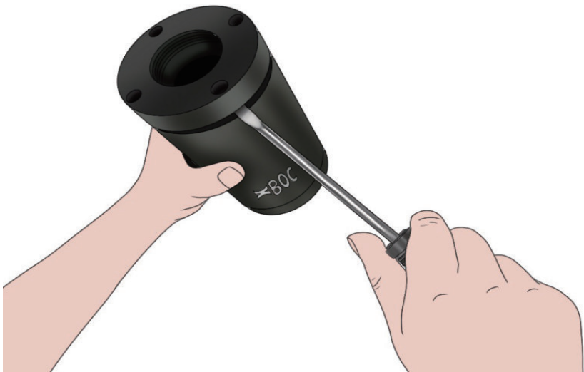
2. Use a flat screwdriver to pry the valve sokcet out
