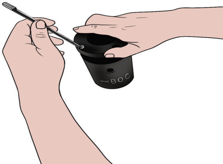
8. Fix the valve socket with screws, and tighten the screws cross-stitch.
