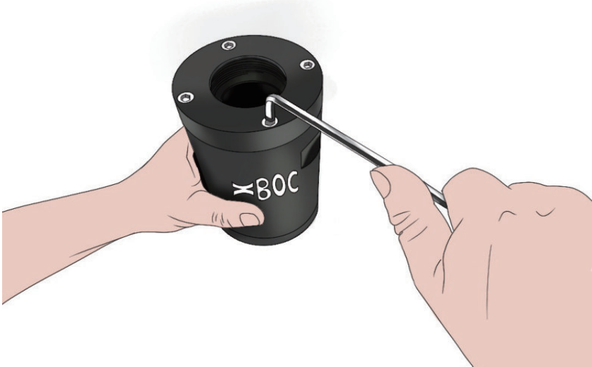
1.Remove all screws with a hex wrench
